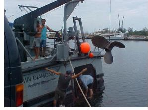
locals was down early the next day ready for the job. After putting and explosive charge around she shaft and setting it off the prop was ready for removal. The process of reshaping the prop took less then a week and we were ready for the first trip out to the site.
